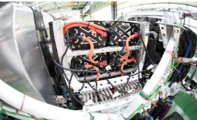
Fig. 5 Photo of module installed in Dakar HEV (Material provider: Hino motors)
