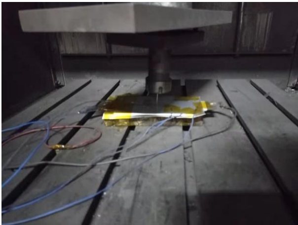
Fig. 4 Schematic of fine nail superficial penetrating of power batter
