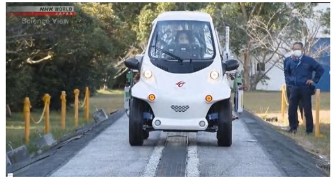
Fig.3 e-mobility on the electric road at TUT 10)
