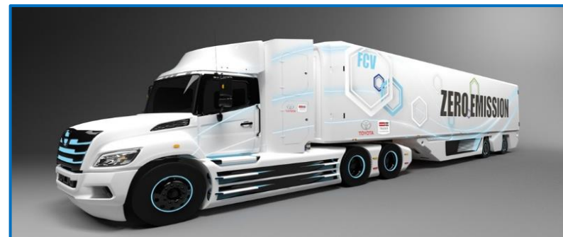
Heavy-duty FC truck based on Hino XL series for the US market, using Mirai’s stacks. The road test began in 2021.
