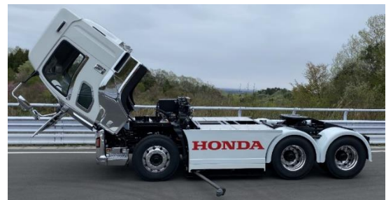
Fig.11 Dynamic Charge Power Unit Layout (6×4 Tractor)
