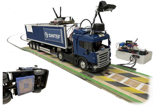
Fig. 1. Picture of 1:14 scale autonomous truck model with camera-based path tracking functionality when passing a road-side coil section for DWPT, with a closer view of the on-board coil shown in the lower left side the figure.
