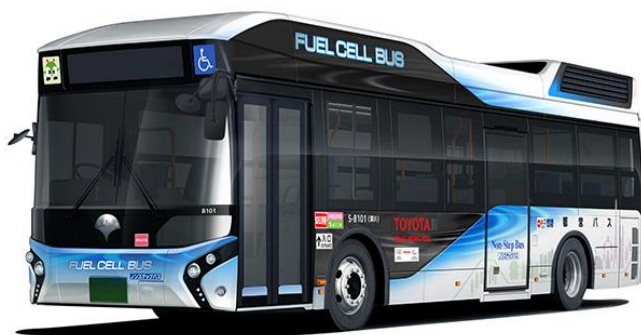
FC bus, “Sora” intraduced in Tokyo, in 2017, Feb., using two Mirai’s FC stacks, Drive range: about 200 km
