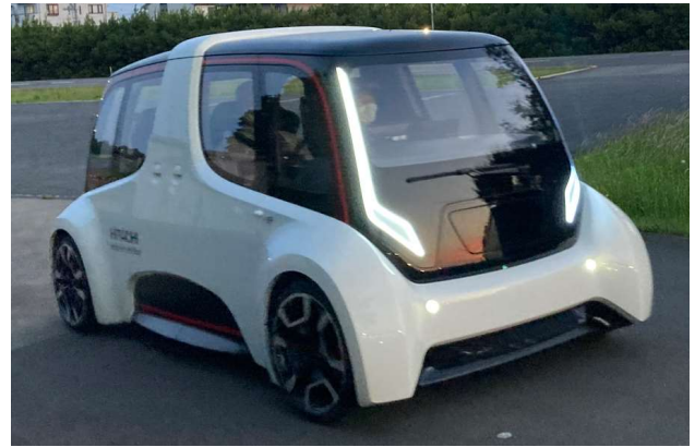
Fig. 9. EV prototype with in-wheel motor.
