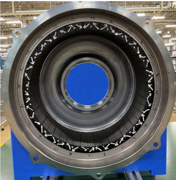
Figure 11: Rotor with an Array Magnet
