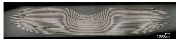
Fig. 3 Cell-center cross section obtained using digital microscope.
