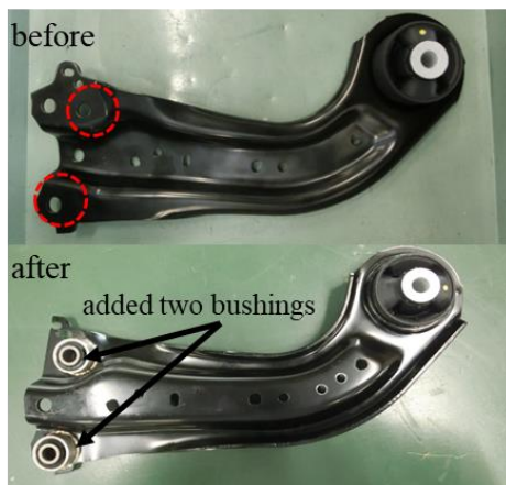
Fig. 18 Adding two bushings to the trailing arm
