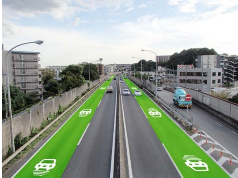
Fig. 1 Concept of our WPT roadway system.
