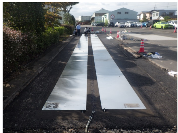
(d) Transmitting electrode on the bituminous stabilized material
