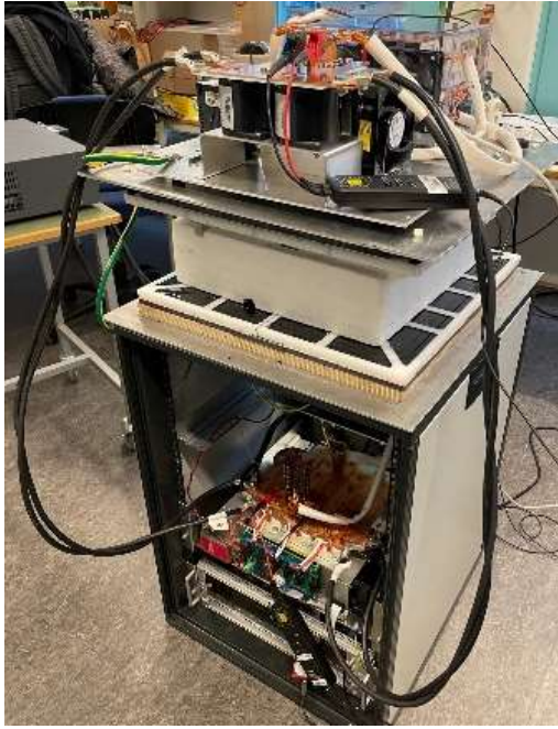
Fig. 7 Experimental setup, including coil assemblies, resonant capacitors, converters.
