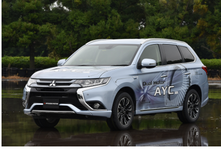
Fig. 15 Experimental vehicle equipped with TDA-TVD. TDA-TVD drives rear wheels using two electric motors.
