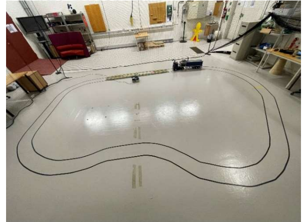
Fig. 8. Photo of the truck operating on the marked test track with the DWPT system
