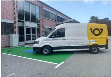
Fig. 4: INTIS' Stationary Wireless Power Transfer System (Slovenian Post, 2022), 22kW, 85 kHz.
